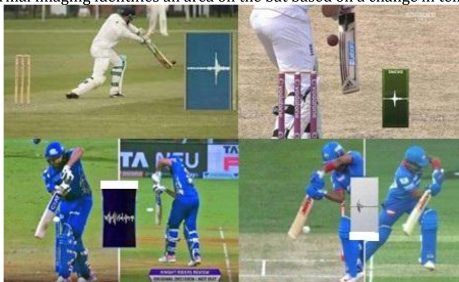
Fig. 3. A spike is identified by the snickometer by means of the sound waveform as the ball is crossing the bat.
